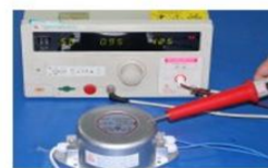
Spot test Waterproof transformer detection
